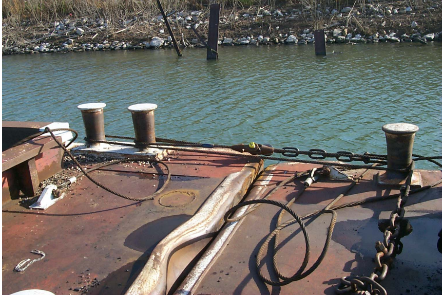
Figure 5.18. Typical port lashing with clevis load cell
