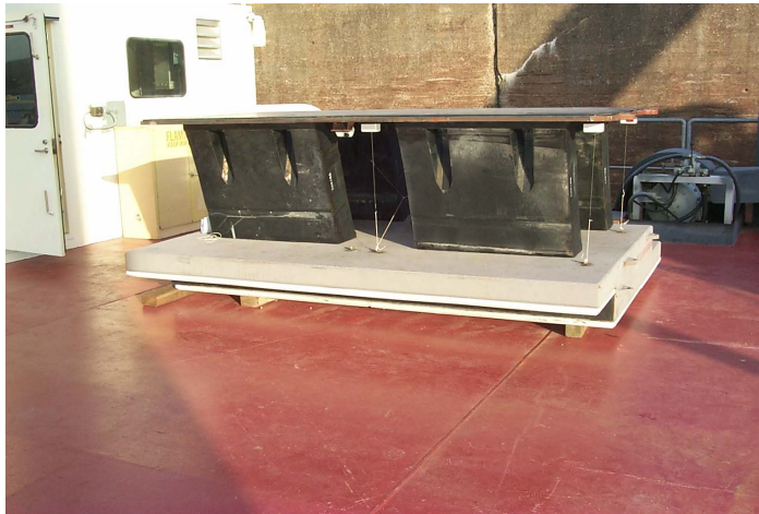
Figure 6.2. Prototype fendering segment—side view
