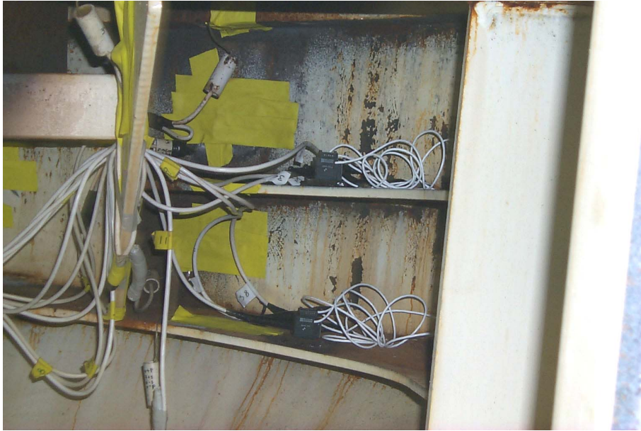
Figure 5.5. Accelerometers on gussets under deck in impact corner
