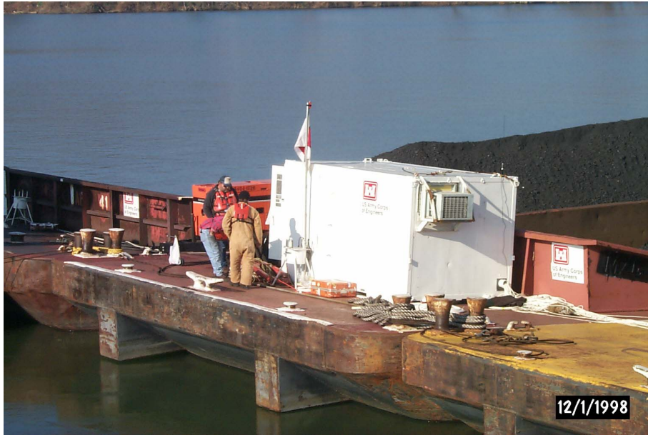
Figure 5.1. Onboard instrumentation enclosure on middle lead barge (Note: barge impact corner is just to the right of the picture)
