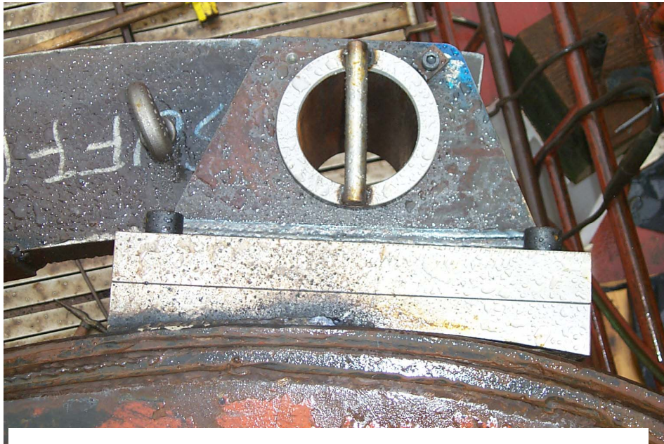
Figure 5.10. Clevis beam load beam (Note: Barge mounting plate is against barge; next is the vertical clevis mount, followed by horizontal clevis mounts. The load beam is under the clevis and runs to the left. The instrumented clevis pin was not inserted at this time to avoid damage during installation of load beam)
