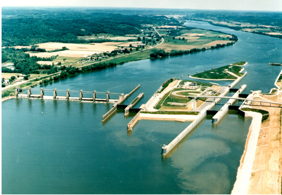
Figure 3.1. Aerial view of Robert C. Byrd Lock and Dam (Old Gallipolis Locks are adjacent to the dam near the middle of the picture)
