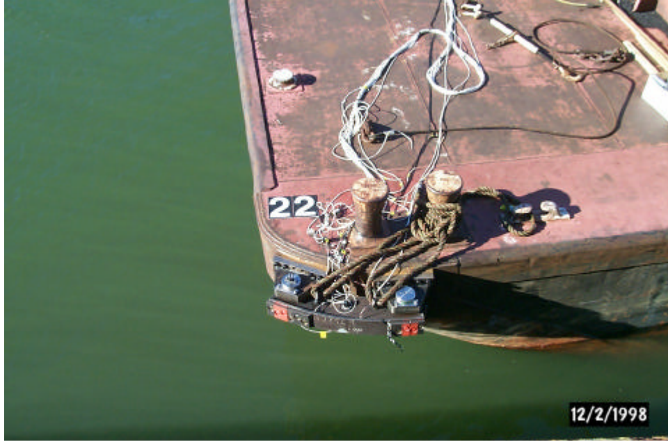
Figure 3.1. Instrumented circular arc beam (bumper)
