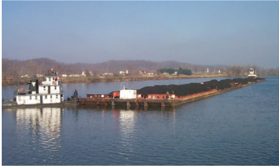
Figure 1.2. Fifteen-barge tow configured for impact experiments
