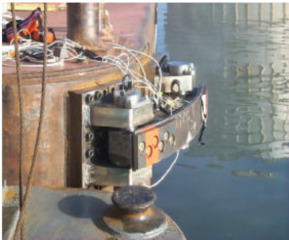
Figure 1.4. Load bumper mounted to the front barge corner
