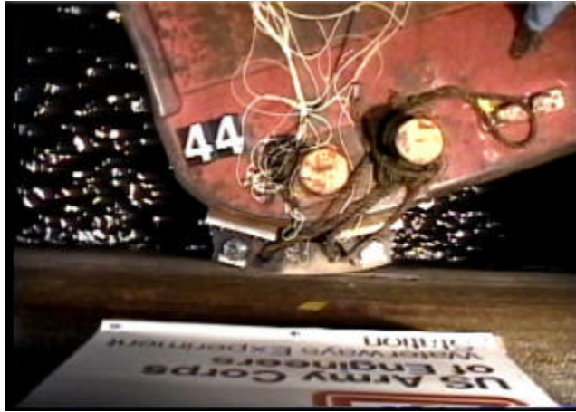
a. Overhead photo of barge with bumper about to impact the lock wall
