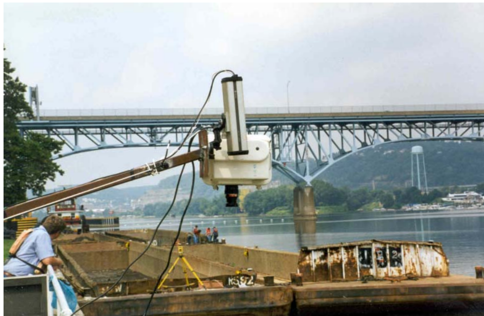
Figure 18. High-speed camera and video camera overlooking impact point
