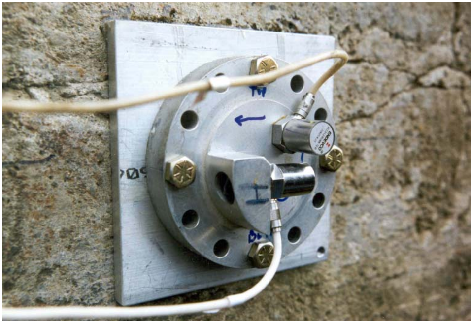
Figure 16. Biaxial accelerometers on lock wall
