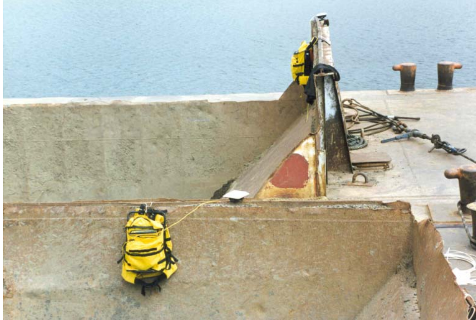
Figure 17. DGPS antennas and recorders on barges
