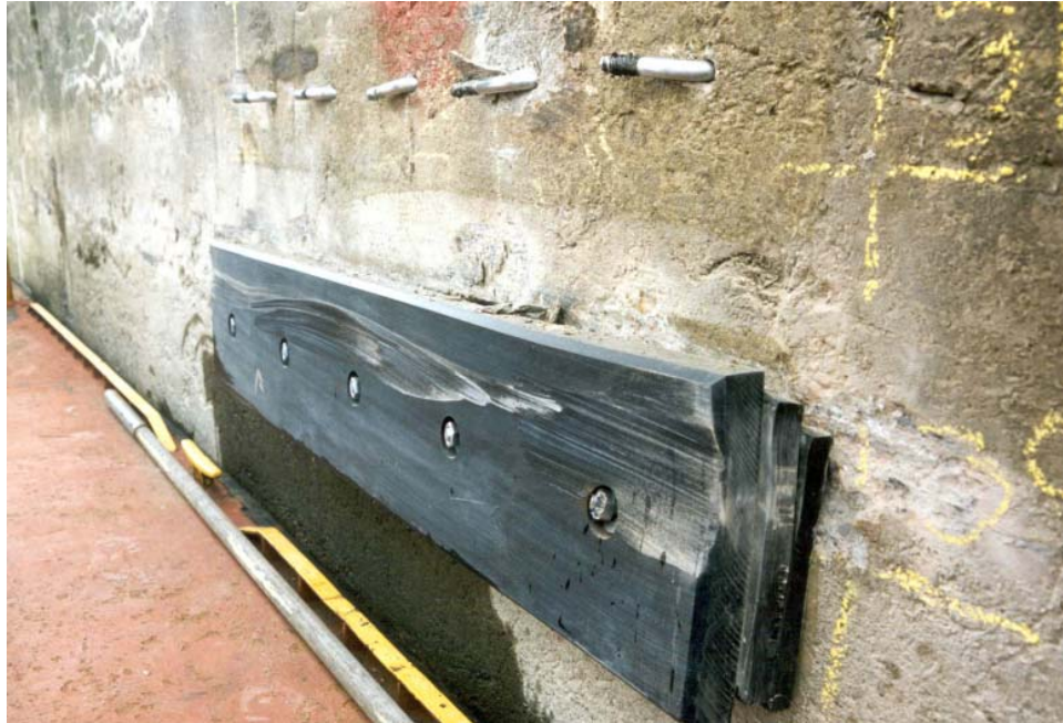
Figure 23. UHMW bumpers after Experiment 29
