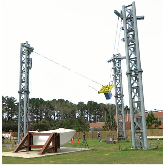
Figure B.3 FDOT pendulum impact facility in Tallahassee, Florida (Source: Kantrales et al. 2015)
