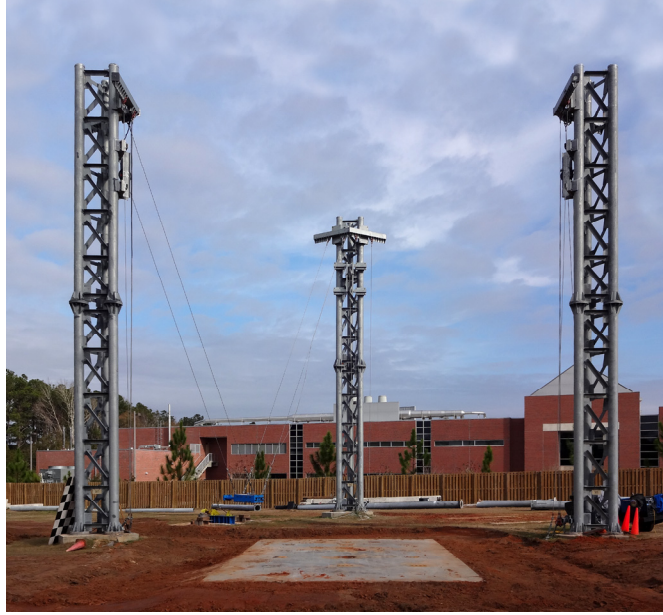
Figure 3.1 Impact pendulum at M.H. Ansley Structures Research Center in Tallahassee, FL
