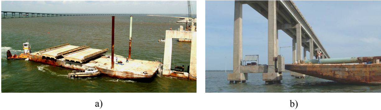
Figure 2.3 Full-scale barge impact experiments at St. George Island, Florida: a) Stand-alone pier impact (superstructure removed), and b) Intact bridge impact (Consolazio et al. 2006)
