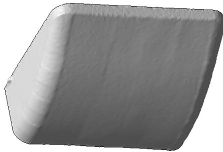
Figure 7.34 3D scan of undeformed replicate barge bow (prior to flat-faced nose test series)
