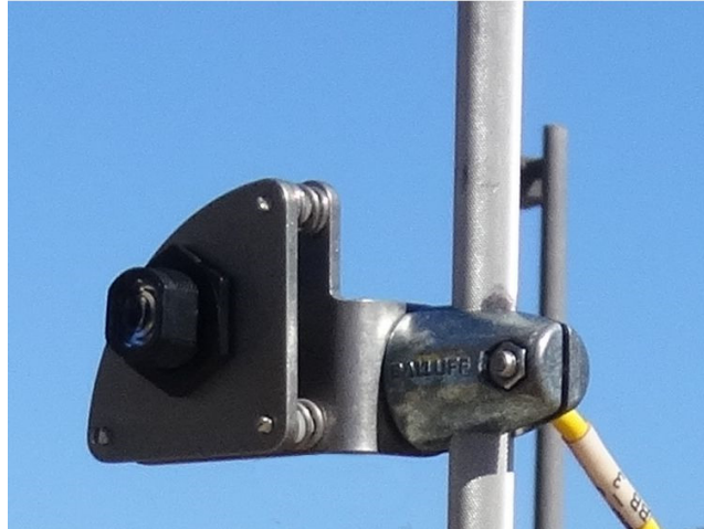
Figure 6.14 Optical break beam sensor mounted on stand
