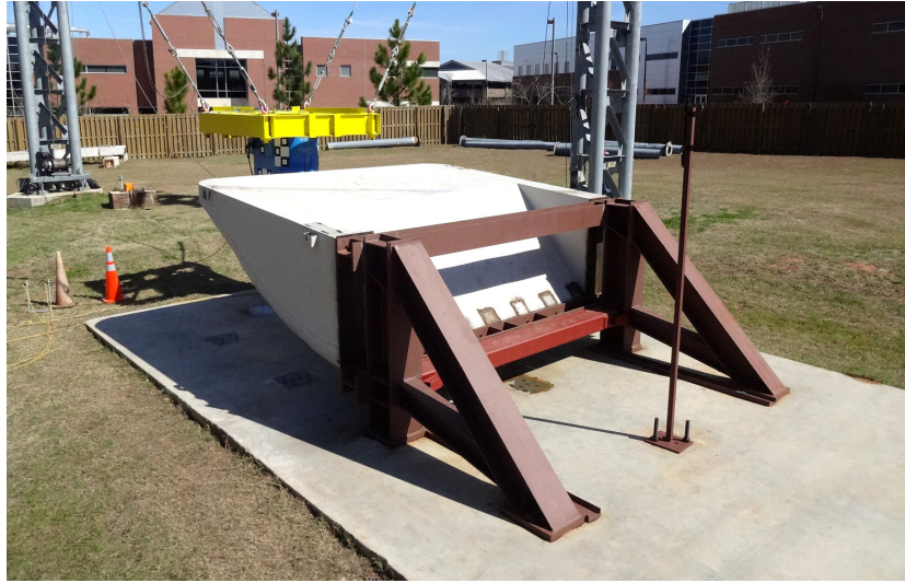
Figure 6.2 Photograph of test setup for barge bow experiments
