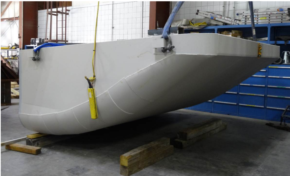
Figure 6.4 Fabrication of replicate barge bow model: a) Exploded view of replicate barge bow; b) Replicate barge bow during fabrication; c) Completed replicate barge bow
