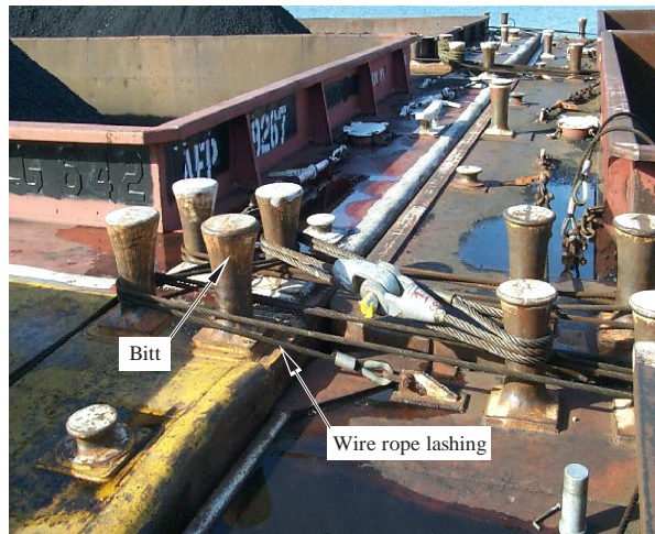
Figure 2.9. Typical lashing configuration on barge flotilla
