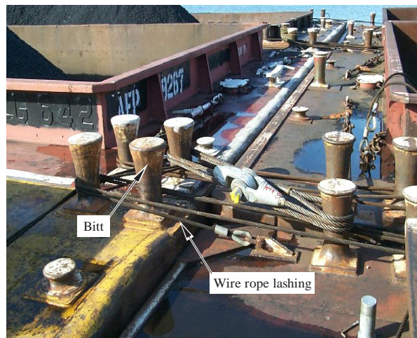
Figure A.1. Typical lashing configuration on barge flotilla
