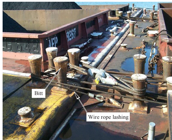
Figure 2.19. Typical lashing configuration on barge flotilla
