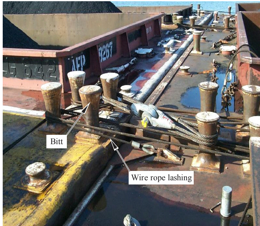
Figure 2.10. Lashing configuration on barge flotilla
