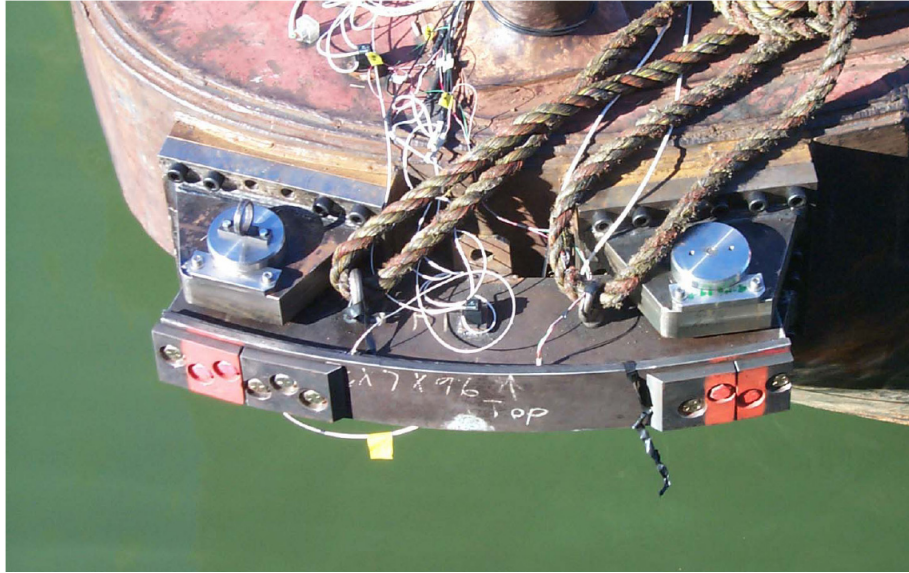
Figure 4.4. Load-measurement system (beam, shear pins, and clevis mounts) attached to corner of barge (Photo credit: US Army Corps of Engineers)
