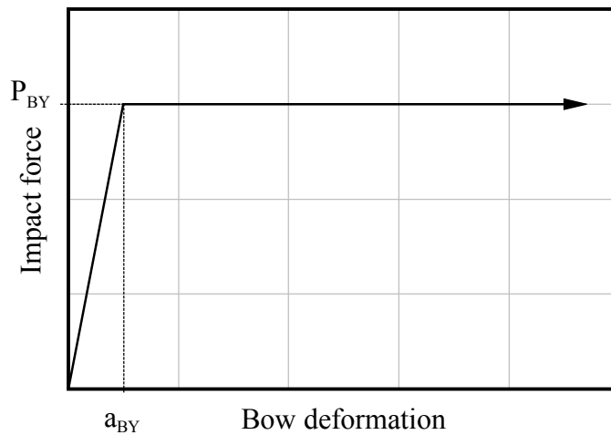
Figure 4.24 Elastic-perfectly plastic barge bow force-deformation curve
