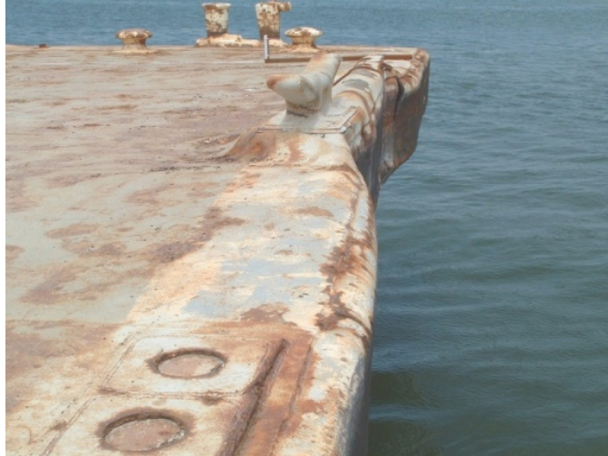
Figure 7.10 Permanent deformation of barge bow resulting from series P1 tests
