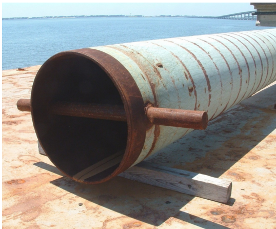
a) Lifting posts at top of spud
