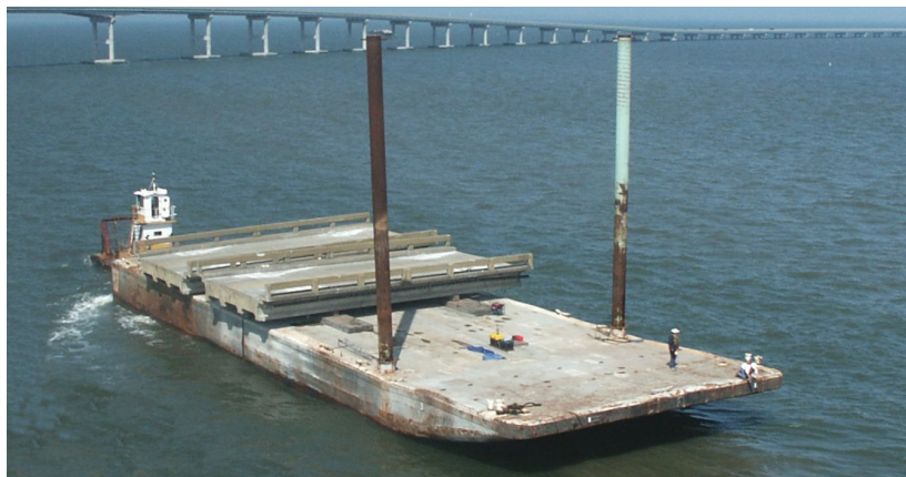
Figure 5.2 Test barge with payload as used in series P1 tests
