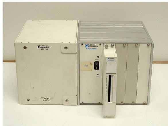
Figure 6.11 Data acquisition chassis configuration used on barge
