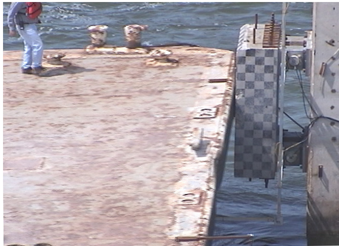
a) Barge bow parallel to impact block (head-on impact) during test P1T4
