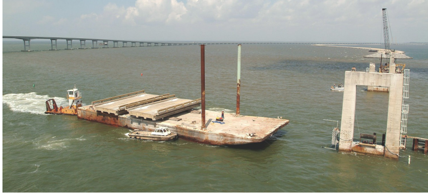
Figure 5.4 Test barge propelled by pushboat and winch cables, and guided by helper boat during test series P1
