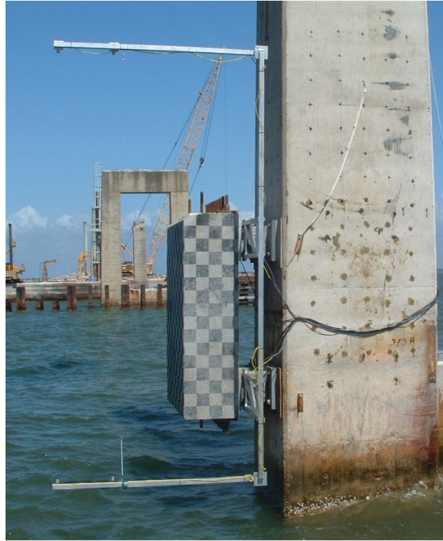
Figure 6.20 Break beam sensors installed on aluminum bracket adjacent to impact block
