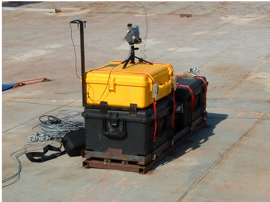
Figure 6.18 DAQ/DC/GPS cases and video camera mounted to the barge deck through a shock isolation sled
