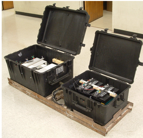
Figure 6.16 DAQ and DC cases connected together and placed on shock isolation sled
