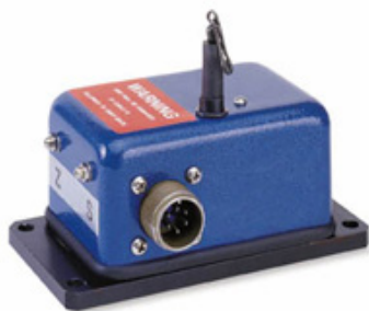
Figure 6.34 Displacement transducer (individually and as installed on timber platform)
