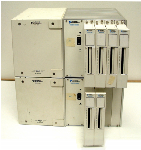
Figure 6.10 Data acquisition chassis configuration used on piers
