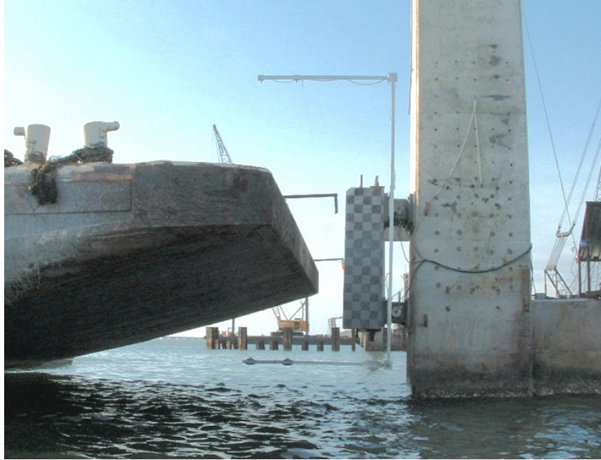
Figure 6.22 Test barge nearing contact with impact block
