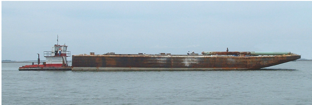
Figure 4.1 Construction deck barge used to conduct impact tests
