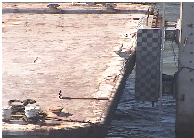
b) Barge bow not parallel to impact block (mildly oblique impact) during test P1T5
