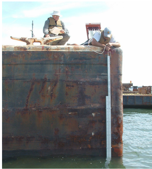
Figure 4.9 Measurement of barge draft
