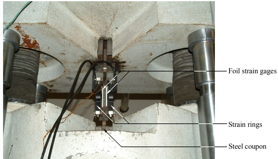
Figure 6.36. Axial loading of a steel coupon instrumented with strain rings and foil strain gages
