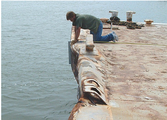
a) Positioning tape rule and rigid square at bow
