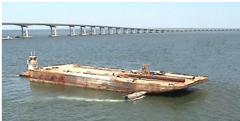
Figure 4.7 Empty-barge condition used during tests on Pier-3
