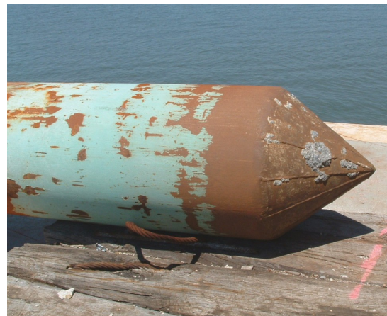
b) Pointed tip at bottom of spud
