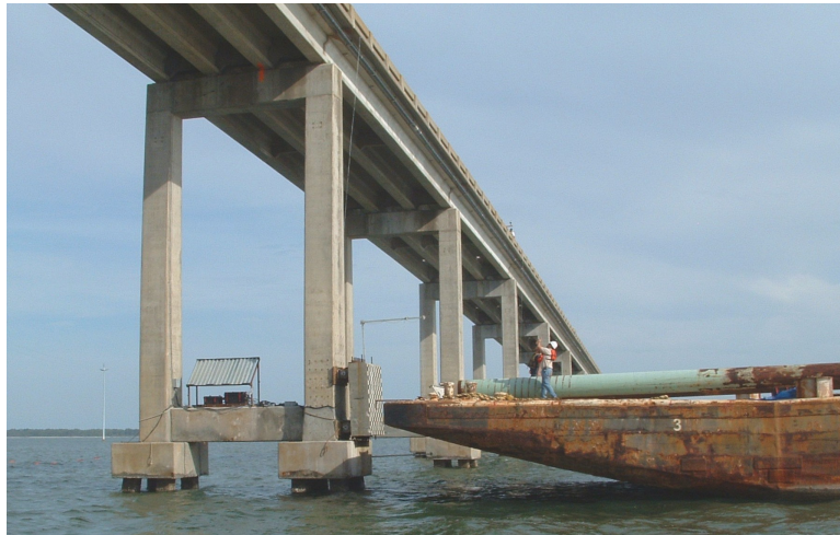
Figure 5.7 Test barge propelled into the bridge at Pier-3 during test series B3
