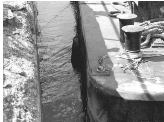
b) Sensors at impact corner of barge
