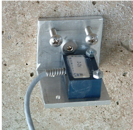
Figure 6.28 Accelerometer mounted to vertical concrete pier surface
