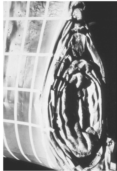
b) Permanent deformation of ship bow model after test
