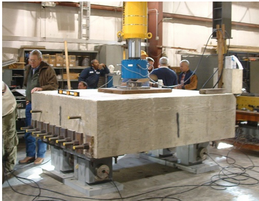
Figure 6.26 Laboratory testing of an impact block and load cells
